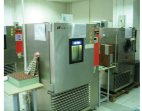
Environmental Test Chamber for Product Burn-In
